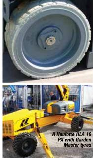
Another option is solid tyres and more recently aperture tyres with a network of openings through the tyre wall to try to emulate the cushioning effect of a pneumatic tyre while eliminating punctures.
