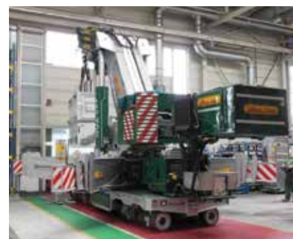
The World Power ER 450.000 L-8 can also be mounted on a compact five axle trolley-type chassis for use in industrial applications.
