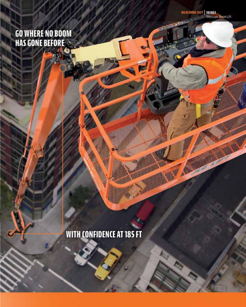
INTRODUCING THE WORLD'S TALLEST SELF-PROPELLED BOOM LIFT. The new 1850SJ has more reach, better stability and a larger work envelope than any lift in its class. Get up to 19 stories of working height and an innovative chassis that can be extended front and back. Featuring 1,000 lb/500 lb platform capacity, the 1850SJ is the most powerful boom in the industry. Transport with ease in a regular size trailer - no oversized load permit needed. Learn more at www.lig.com/en/1850sj-1.
