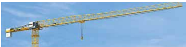
The new tower crane has 15 percent better capacities and can now lift 2,100kg at its maximum radius of 60 metres.
