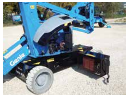
Genie is currently working on a quick swap over system for the battery packs for multi-shift applications.
