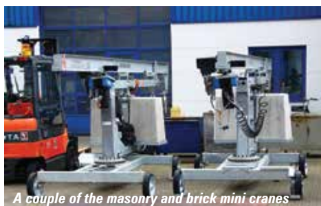
A couple of the masonry and brick mini cranes
