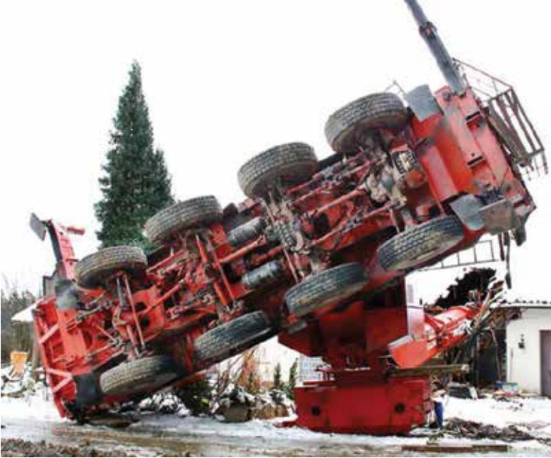
New outrigger monitoring standards will reduce the number of short rigged incidents.
