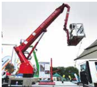
The TU 285 has 20.5 metres outreach and variable jacking.
