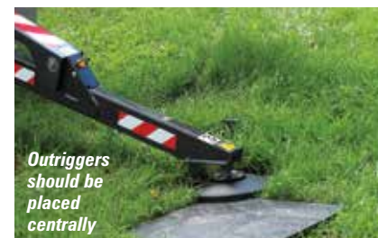
Pads should be rigid and not deform
