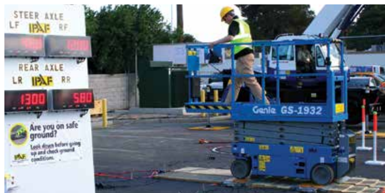
IPAF's demonstration at Conexpo 2011 revealed just how much pressures can vary between the wheels of a platform.
