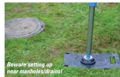
Outriggers should be placed centrally
