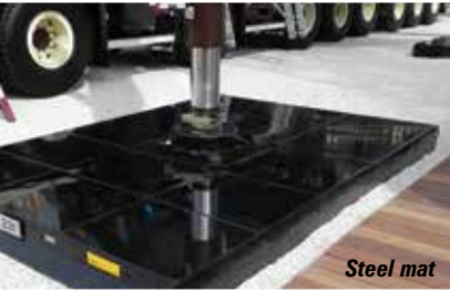
Outrigger located within the pad
