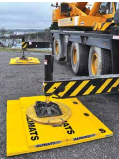
Alimats interlocking modular load spread system.
