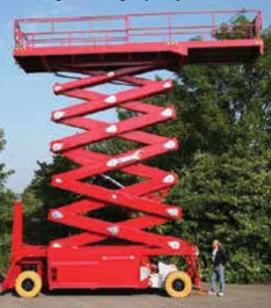
PB Liftechnik's 27.25m working height 1,000kg capacity PBS270-24E
