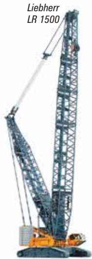
The all new LR 1500 is said to be a 500 tonne capacity crane with the dimensions and weight of a 400 tonner
