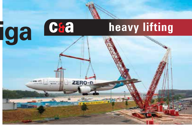
Sophisticated hanging gear: the combination of cross and spreader beams was able to adjust the angle to the appropriate centre of gravity using an electric chain hoist.
