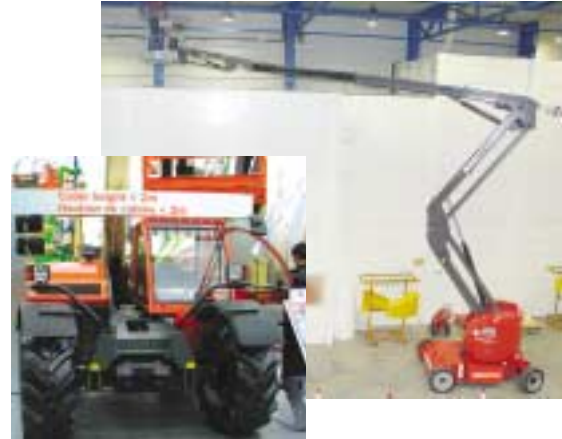
JLG offer a low overall height version of its 266 telehandler, dubbed the Lo Pro, it will pass under 2 metre bar.
