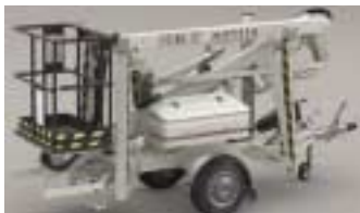
A telescopic upper boom gives the Matilsa Parma 120T a very short travel length
