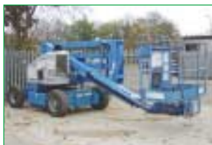
SELF PROPELLED TELESCOPIC 1995 GENIE Z 45/25 Bi-fuel. 15.5m. metre working height (51ft.). Kubota diesel and battery bi-fuel.
