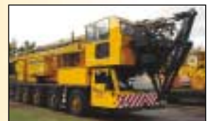
Spierings SK598 Year 2001/3. Capacity 8 tonnes. Mobile Tower
