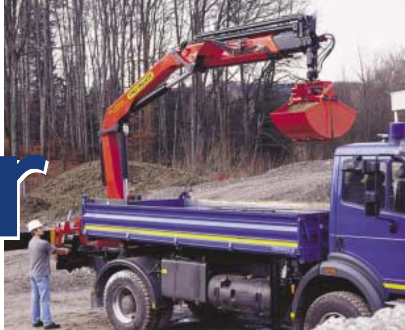
Lorry loaders that are fitted with grabs will have had much more use than those with hooks.
