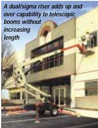
Articulating-telescopic machines like this Genie are great when you need to get up and over
