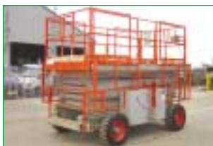
SELF PROPELLED SCISSOR 1997 SKYJACK 8841 14m. working height (47ft.). 2WD, Twin Extending Decks.
