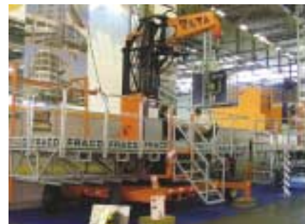
Fraco exhibited a heavy duty mast climber with heavy jib, alongside a light towable mast climbing platform.
