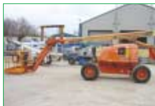
SELF PROPELLED TELESCOPIC 1999 JLG 600AJ 20m. working height (66ft.) Articulated Jib.
