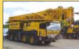
Liebherr LTM1090/2 Year 1997. Capacity 90 tonnes. All Terrain
