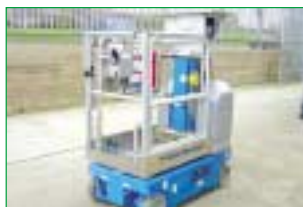
PERSONNEL PLATFORM 2005 GENIE GR12. 5.58m. working height (18ft.). Compact design, Dual voltage charger.
