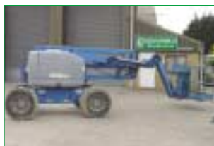
SELF PROPELLED TELESCOPIC 2001 GENIE Z45/25J 4X4 15.9m. working height (51.6ft) 4WD Rough terrain, Fly jib, Foam tyres
