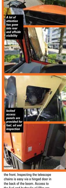
the fuel and hydraulic oil filler are placed next to the cab behind locked
