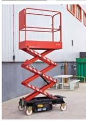
The expanding ELS Makine access range includes this 5.3 metre working height Junior 5.5 push around.
