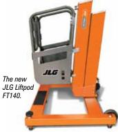
JLG is obviously committed to this concept and launched a larger generation Liftpod - the FT140 - at Conexpo earlier this year. Retaining the key Liftpod features, it is simple to assemble, operate and transport and has the same 150kg capacity, but offers a significantly improved working height of iust over six metres. The FT140
