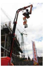
Cormidi KB23 showing off its access jib attachment. The crawler crane in the background was not part of the show and just happened to be working on an adjacent site.
