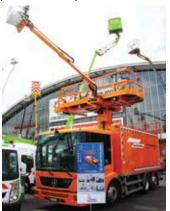
France Elevateur showed its 105 PTO-2 - one of seven sold to Kummler+Matter for working on the Swiss tram system. The unit has a five person capacity with two booms either side of the main platform.
