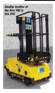
working height of 5.5 metres and a moveable loading platform capable of carrying up to 90kg for stock picking duties.
