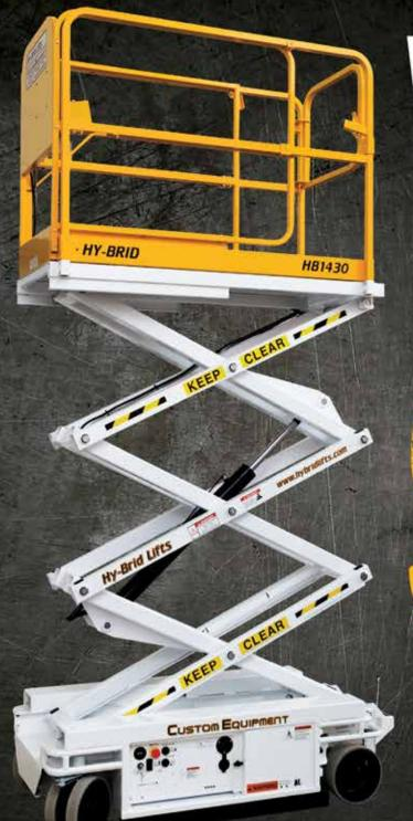
Hy-Brid low-level scissor lifts might be compact, but they deliver in huge ways. Light weight, yet high capacity. Ample platform space, yet small enough to maneuver into elevators and through doorways. Low stowed heights, yet 20-foot working heights. All resulting in versatility thats needed from start to finish on every job.
