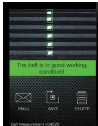
Determining belt wear.
