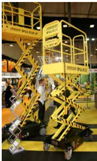
The 5.1 metre working height X3X-SP, is 760mm wide, weighs 496kg and features a 1.65 metre platform length and a 400mm deck extension.
