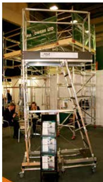
As well as its range of PAS 250 certified podiums Euro Towers showed a prototype of its self-erecting Z-Fold tower. Designed to be erected entirely from the ground the 4.2 metre working height Z-Fold easy folds down to allow passage through standard doorways and transportation in a large estate car.
