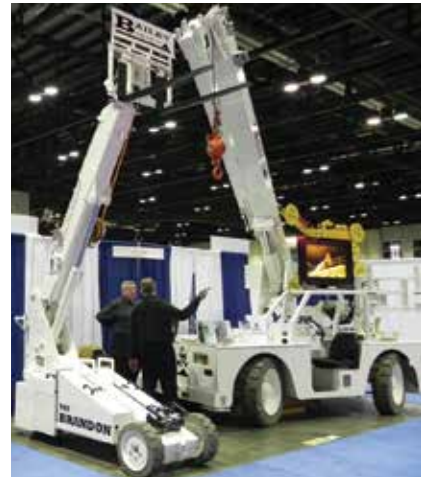
The newly formed Bailey Crane showed a new 8 tonne hybrid carry deck crane.
