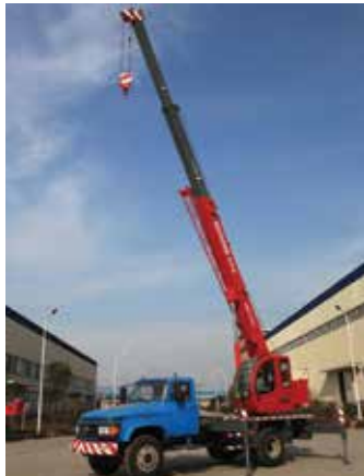
The eight tonne Manitowoc Dongyue GT8 truck crane.
