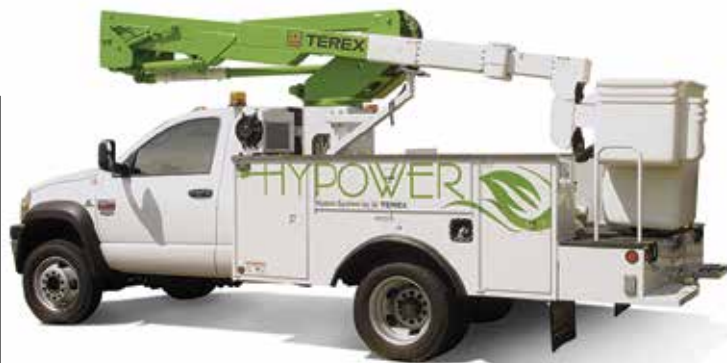
An increasing number of utility type vehicle mounted lifts are equipped with lithium hybrid power packs.
