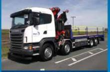
New Scania 8x2 G400. Fassi 455 remote crane with cheese wedge body
