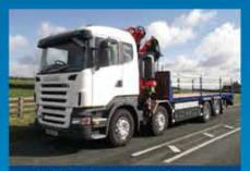
2010 8x2 Scania G400. Fassi F275 remote with cheesewedge body. 17 ton payload.
