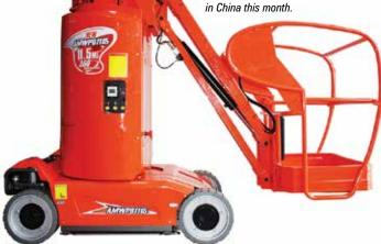
the same as most sub 12 metre models - with an overall length of 2.56 metres and an overall stowed height of 1.97 metres - both slightly more compact than the Star 10 and quite a bit more compact than the ATN1100R. Gross weight is 2,850kg - around 120kg heavier than the Star 10 but lighter than the Piaf 1100R - although it is not clear if this includes the optional overload cut-out system, a legal requirement in Europe.
