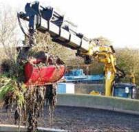
The ACC 2050 working with the fully hydraulic rotating rehandling grab
