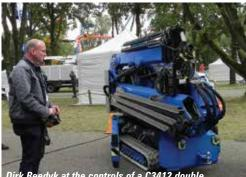
Dirk Reedyk at the controls of a C3412 double articulated mini crane with 4.25 tonnes maximum capacity and 21.5 metres maximum height
