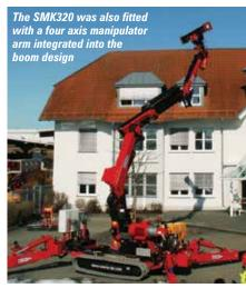
working height of 22.5 metres, an outreach of nine metres and a platform capacity of 200kg, or 12 metres with 80kg. The lift also provides around seven metres of horizontal outreach at an up and over height of around 14 metres.
