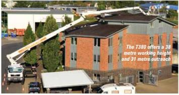
German truck mounted lift manufacturer Ruthmann has unveiled its new 38 metre T380 truck mounted lift, on a two-axle 18 tonne chassis. The T380 offers an outreach of 31 metres, a 180 degree articulating jib and a maximum platform capacity of 600kg. Ruthmann will also announce the launch of the 63 metre T630 in the coming weeks.
