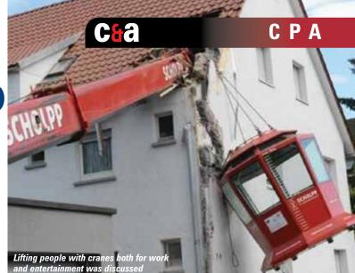
requires lifting equipment used to lift people should be thoroughly examined at least every six months. The HSE has confirmed that this applies to elevating cabs on cranes. The rest of the crane - assuming it is not used to lift people with a manriding basket - can still be examined every 12 months.
