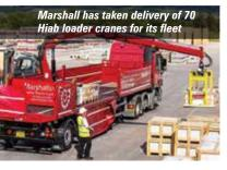
The new cranes have been fitted with Hiab's Operator Protector System and can be operated either with the remote controller or from a raised standing platform fitted to the crane. The company said its drivers particularly like the ease-of-use, responsiveness and precision of the radio remote controls.
