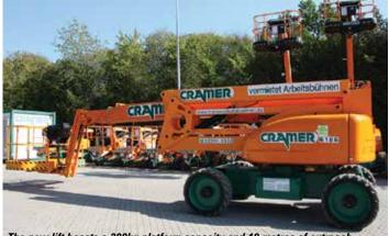
The new lift boasts a 280kg platform capacity and 19 metres of outreach
