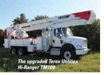
Terex Utilities has launched an upgraded version of its Hi-Ranger TM100 telescopic aerial and material handling device. The new model has a lower overall stowed height of 3.9 metres, a new outrigger and sub-frame configuration that reduces the vehicle's weight - allowing installation on a wider range of standard trucks, including a 6x6 chassis and/or increased payload capacity.
