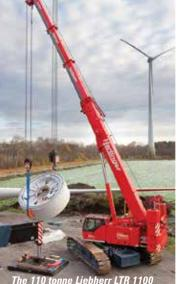
to the thoroughbred All Terrain booms installed on some crawler models. In basic trim with one metre wide tracks the unit weights around 90 tonnes and is capable of assembling itself without the need for an auxiliary crane.
