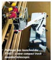
**Palfinger Platforms has launched** a new 13.5 metre telescopic compact truck mounted platform - the P140T.
