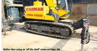
Rather than using an 'off the shelf' undercarriage, the ACC 2050/1 has a specifically designed chassis with three position outriggers front and back
