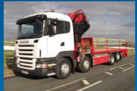
2010 Scania 8x2 R420. Fassi 455 remote crane with choice of flat or cheese wedge
