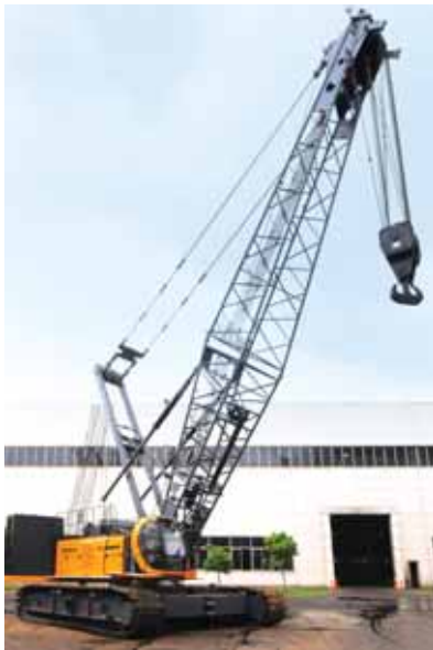
Sany America has added a new crawler crane to its line-up with the 165 ton (150 tonne) SCC8150.
