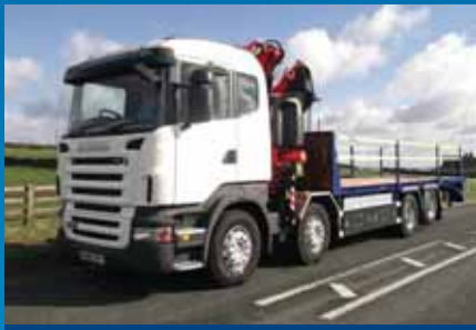
2010 8x2 Scania G400. Fassi F275 remote with cheesewedge body. 17 ton payload.
