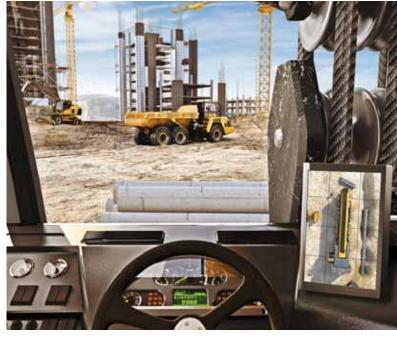
A bird-eye view of the vehicle and its surroundings are displayed on a screen in the cab.
