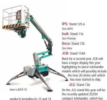
products including its 12 and 14 metre IT10090 and IT12133 self-propelled scissor lifts. With platform capacities of 300kg and 350kg respectively, the battery powered lifts include a roll-out deck extension of 1.4 metres. Also on the stand will be the 15 metre IM R 15 tracked spider lift which offers an 8.7 metre outreach and its 5.2 metre Easy Up 5 SP self-propelled micro scissor lift.
