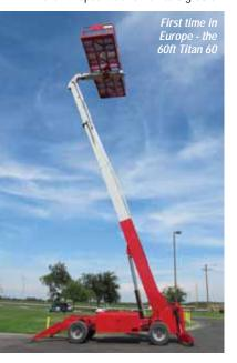
Titan 60 scissor type platform on a boom which has the capacity of a telehandler, following the success of the original Titan 40. The company will also have a good deal to say about its new European distribution operation and you may have a chance to see its unusual Crossover scissor products with special offset platform as well as hear about its recently launched big RT scissor lifts.
