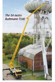
mounted on a 26 tonne chassis - the second model in the company's recently completed Height Performance range.
