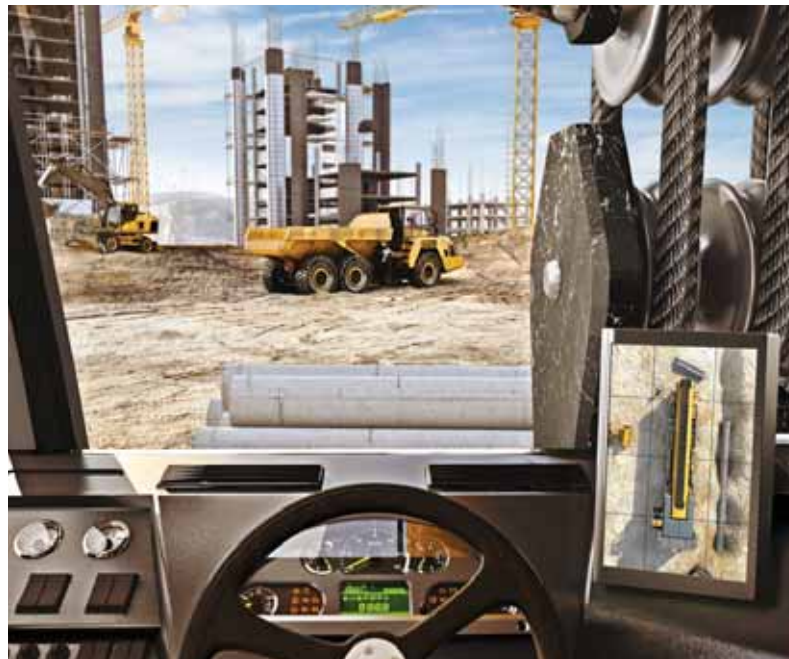
A bird-eye view of the vehicle and its surroundings are displayed on a screen in the cab.
