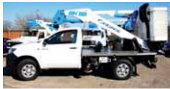
The 13.5 metre Hilux A314 offers a 6.5 metre outreach.
