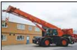
2008 Tadano GR-700EX - 70t Rough Terrain Crane, 44m Boom + 17.6m Fly
