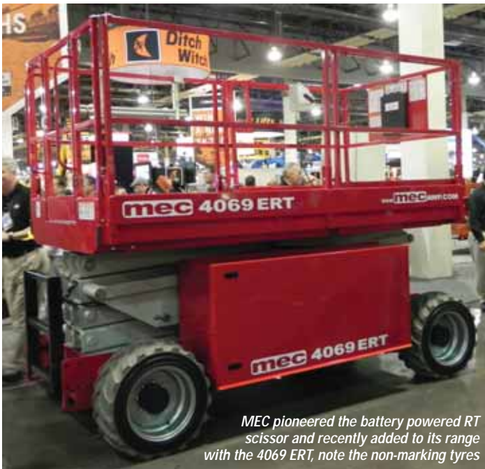
MEC offers an offset deck design on its ERT and Crossover models, which gives users a platform that extends to the full chassis width on one side and incorporates an inboard sheet or tube rack on the other side.
