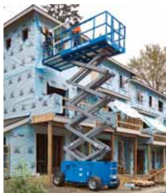
Battery powered Rough Terrain scissor lifts are gaining in popularity - the GS4069DC boasts the same performance as the diesel powered models.
