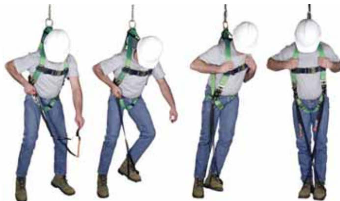
Suspension loops can be used to alleviate the effects of suspension trauma.
