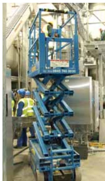
Most electric scissor lifts are slab models with seven to 11 metres working heights
