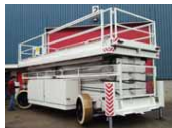
Holland Lift introduced a more compact version of its 34 metre working height electric scissor lift.
