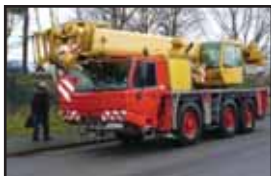
2004 Tadano Faun ATF 45-3 - 45t All-terrain Crane, 34m Boom + 15.2m Fly
