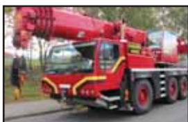
2004 Liebherr LTM 1055 - 55t All-terrain crane, 40m Boom
