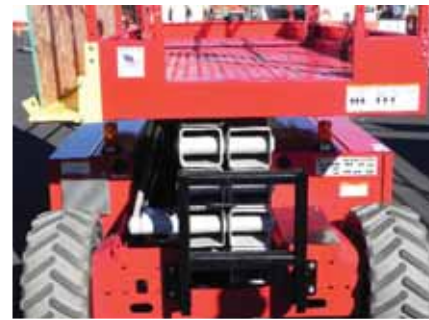
MEC offers an offset deck design on its ERT and Crossover models, which gives users a platform that extends to the full chassis width on one side and incorporates an inboard sheet or tube rack on the other side.
