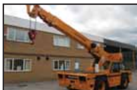
2010 Broderson IC-200-3G 13.6t Pick & Carry Crane, 15.2m Boom, 7.7t carry deck
