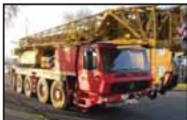
2002 Grove GMK 4075 - 80t All-terrain crane, 43m Boom + 17m Fly
