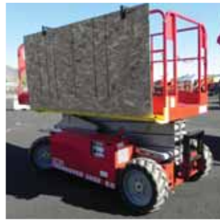
MEC offers an offset deck design on its ERT and Crossover models, which gives users a platform that extends to the full chassis width on one side and incorporates an inboard sheet or tube rack on the other side.
