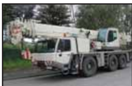
2006 Tadano Faun ATF 60-3 - 60t All-Terrain Crane, 40.2m Boom + 16m Fly
