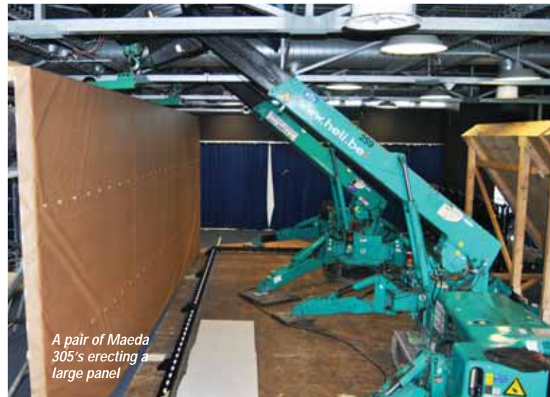
A Bluelift spider lift with winch attachment
