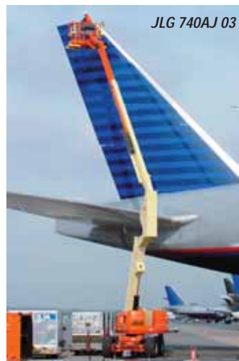
JLG 740AJ allows operators to work outside the basket
