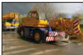
2000 Tadano Crevo TR-200 EXC 20t city crane, 27.5m Boom + 3.5m Fly
