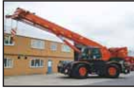
2008 Tadano GR-700EX - 70t Rough Terrain Crane, 44m Boom + 17.6m Fly
