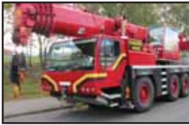
2004 Liebherr LTM 1055 - 55t All-terrain crane, 40m Boom
