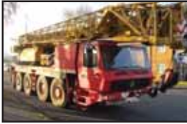
2002 Grove GMK 4075 - 80t All-terrain crane, 43m Boom + 17m Fly
