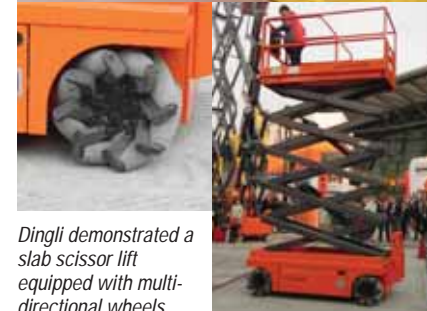
Dingli's new compact - 1.2 metre wide, 16 metre working height slab scissor lift
