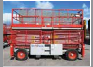
Skyjack SJ-9250 Diesel scissor lift 17.24m/909kg - 2007
