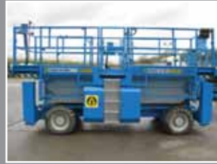
Genie GS-3384 RT Diesel scissor lift 12.06m/1134kg 2005/6/7/8
