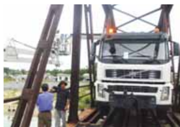
Platform for extending deck units provide a large work/inspection area
