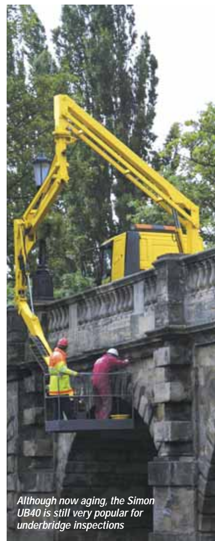
Platform or extending deck units provide platform lengths up to 25 metres
