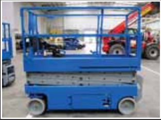
Genie GS-2032 Battery scissor lift 8.10m/363kg - 2005/6
