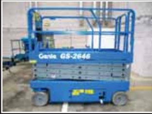
Genie GS-2646 Battery scissor lift 9.92m/454kg - 2005/6/7/8
