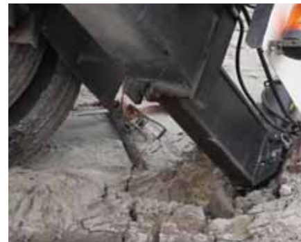
Sand is another No-No - even with its larger fitted pads placing them on soft sandy soil was never going to work.
