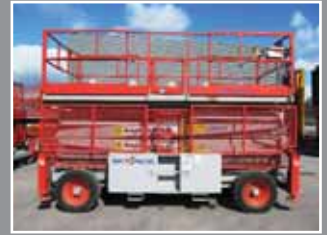
Skyjack SJ-9250 Diesel scissor lift 17.24m/909kg - 2007
