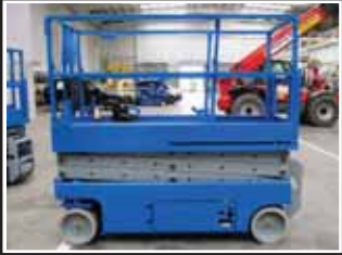
Genie GS-2032 Battery scissor lift 8.10m/363kg - 2005/6
