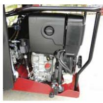
From 2012 Hinowa is introducing a three step automatic setting with speeds of 1,800, 2,200 and 3,600 rpm depending on function demand.
