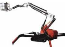
Cormidi main boom and double articulated telescopic jib offers around seven metres of horizontal outreach at an up and over height of around 14 metres.
