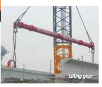
length of 19 metres or 800 tonnes at 14 metres. The beams can be extended in increments of 250mm. Also look for its wire rope slings, shackles and Ekki Hardwood outrigger mats.
