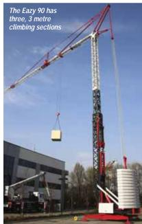
troubleshooting. Jib maintenance or changing the jib configuration can be carried out by lowering the jib to ground level.
