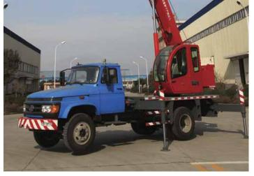
Manitowoc has launched two new Dongyue truck cranes for the local Chinese market. The eight tonne GT8 and 10 tonne GT10A benefit from the improved design and production processes now implemented at the company's plant in TaiAn, Shangdong Province, including the move to Solidworks CAD software, finite element analysis and Design For Manufacture and Assembly methodology.
