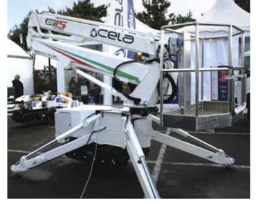
The DT15 is unusual in that it features a two stage highly versatile outrigger system and is lightweight at just 1,550kg.
