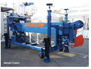
With beam lengths from 2.4 to five metres, the mobile and portable A-Frame crane has a two tonne lift capacity.
