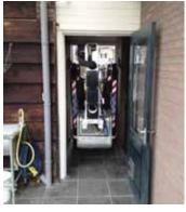
Hoogwerker Centrum realised that the only platform able to fit was a compact tracked spider lift and selected an Oil&Steel Octopussy Classic 1402.
