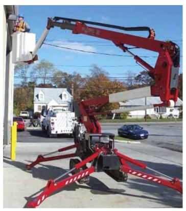
The 17 metre PB18.90.46 is fully insulated to 46KV with special fibreglass sections in the riser and levelling linkage as well as the jib.
