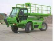
15 metre version of its road-going boom come big RT scissor lift, the MPR15 which is also available with an 18 metre working height. Platform capacity on both is 1,000kg. The company is also expected to show one of its latest Roto 360 degree telehandlers.
