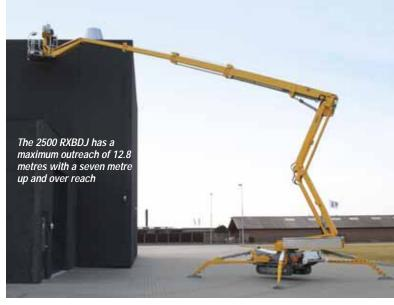
comprises a heavy duty dual arm sigma type riser, four section telescopic boom and a 1.4 metre articulated jib.
