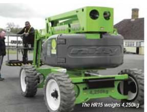
In Europe transportation on 26 tonne delivery trucks should be possible. Power options include diesel 4x2, diesel 4x4 or Hybrid/ Bi-Energy 4x4 with a full battery powered unit possible. Gradeability is 40 percent, platform rotation a full 180 degrees and jib articulation 150 degrees.
