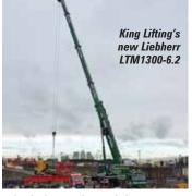
features a single engine which powers both the carrier and the crane superstructure via a combination of mechanical shafts.
