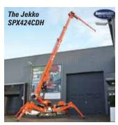
and reach, the overall weight of the machine remains at 2,300kg, allowing it to be towed on a two axle trailer in Germany. The company claims that it is the only crane in its class which can be transported on a 3.5 tonne flatbed trailer.
