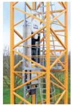
The LiLIP elevator is installed internally on larger tower
