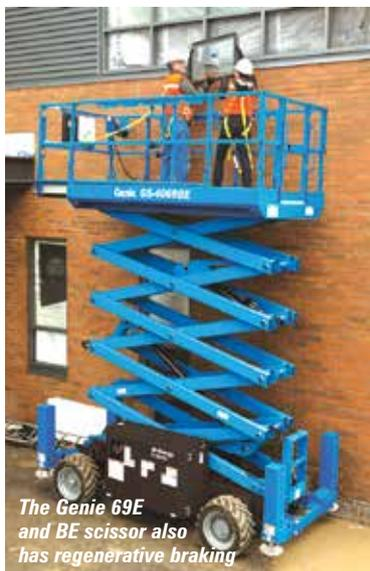
*The Genie 69E and BE scissor also has regenerative braking*
