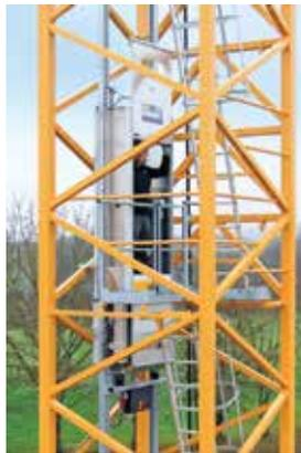
The LiUP elevator is installed internally on larger tower sections.
