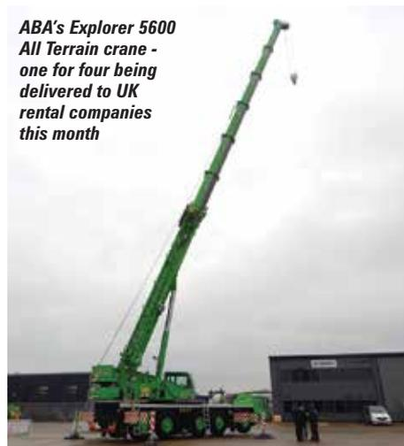
The five axle single-engine Explorer 5600 features a seven section, 68 metre main boom, plus a 21 metre bi-fold swingaway with a 12 metre straight insert, for a maximum tip height of 94.6 metres. Other cranes on display included a 40 tonne AC40/2L City crane for King Lifting, two 60 tonne Challenger 3180s for AB2000 and Sparrow Crane Hire and a 220 tonne Explore 5800 for HTC Plant.
