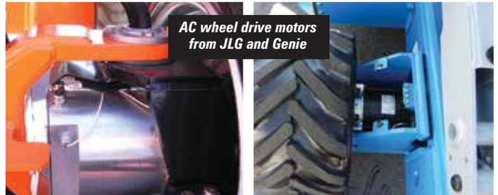
AC wheel drive motors from JLG and Genie
