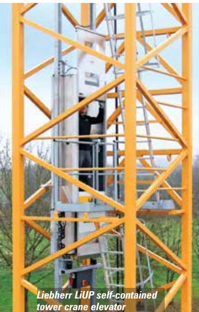
Liebherr LiUP self-contained tower crane elevator
