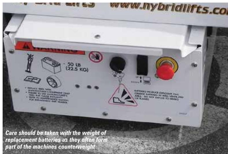
Care should be taken with the weight of replacement batteries as they often form part of the machines counterweight
