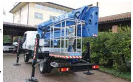
The CTE Z23.2JH platform: caption: The new CTE Z21 and Z23.2JH include a new platform and rotator, new structure and new controls.
