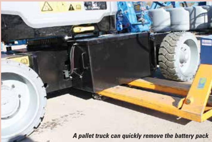
A pallet truck can quickly remove the battery pack
