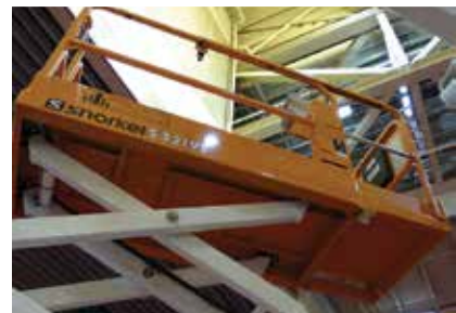
Snorkel's dual component chests and new scissor arm design
