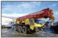
1999 Faun ATF-3 50 Ton All Terrain Crane
