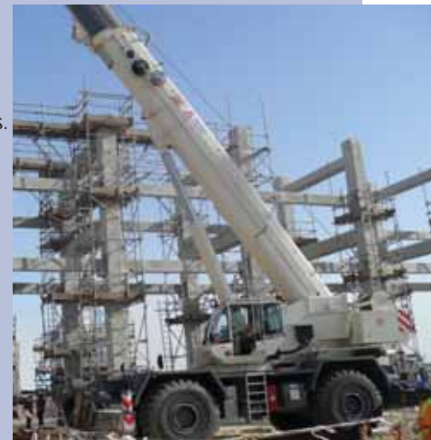
Integrated Logistics Co. KCSC has taken delivery of two 90 tonne capacity Terex RT 100 Rough Terrain cranes in Kuwait to work on maintenance tasks in the petro-chemical and gas refinery sector.
