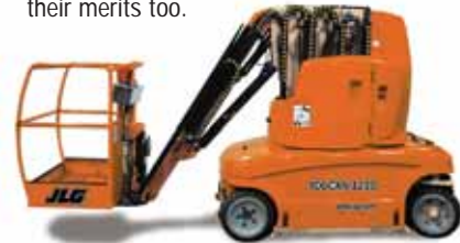
The largest mast booms today are built by JLG with 12 and 13 metre working heights.
