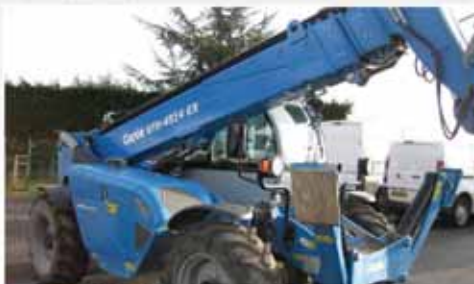
Genie GTH-4514 EX Telehandler from payload 3,5 to 4,5 t and from 13 to 17 m lifting height
