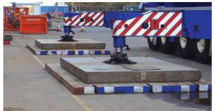
Timber mats are sometimes used under steel to absorb tension.
