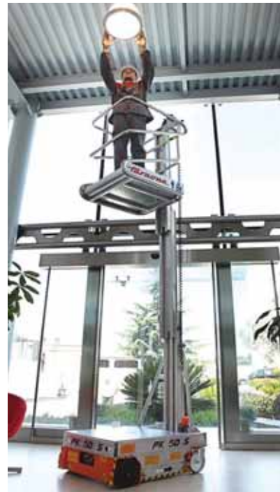
The new PK50S has a three metre platform height and weighs less than 300kg.
