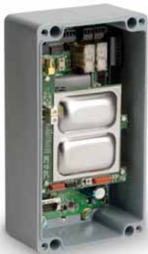
The Windows compatible remote control receiver.
