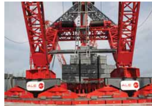
Front view of the AL.SK190 with winches on lower cross beam back mast.
