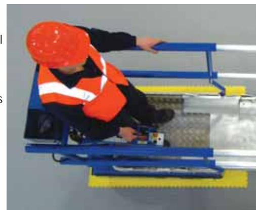
The Nano SP is driven while braced against the guardrails.
