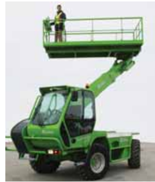
Merlo unveils its MPR 15 and 18 All Terrain big platform aerial lifts using a telehandler boom and a four by two metre scissor lift sized deck.
