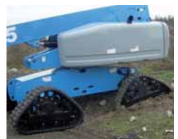
The Loegering crawler units can be retrofitted to a boom lift and then converted back again.
