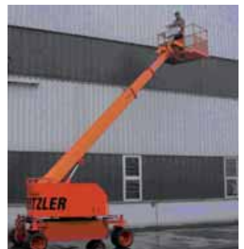
A boom for industry, the unusual 14m Kitzler KIB 24/162T straight boom offers four wheel over centre steering and 500kg lift capacity.
