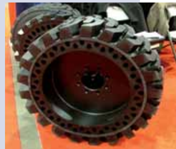
A Solid-flex rough terrain tyre currently used on skid steers will soon be available for aerial lifts.
