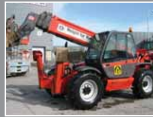
Manitou MT 1740 Telescopic forklift 17m/4 Tonne - 2005
