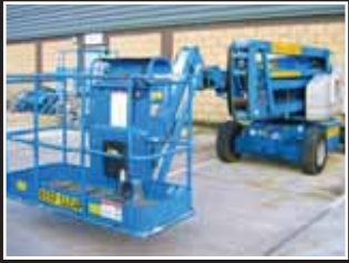
Genie Z-45/25J Bi Articulated boom 15.90m - 2003/4/5/6
