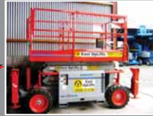
SKYJACK SJ-6832RT Diesel scissor lift 11.50m/386kg - 2007/8
