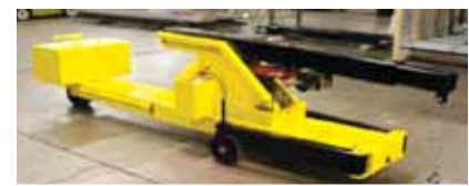
The Smart-Rig crane has decent lifting duties for its size.
