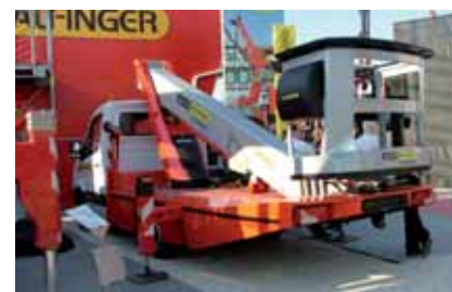
Aluminium and glass fibre keep the weight down on Palfinger's new TA25.
