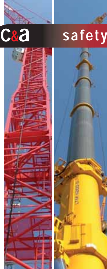
When putting very high booms into the air there might be restrictions as far as 15km from an airfield.
