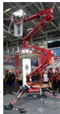
The new 18.8 metre working height spider Lightlift 19.65 has a minimum width of 786mm.
