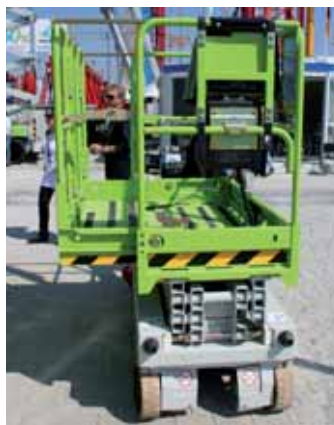
A 360mm side extension is available on Iteco's new 15ft IT4680 M.
