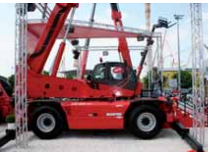
The MRT 3050 has a lift height of 30 metres and maximum capacity of five tonnes.
