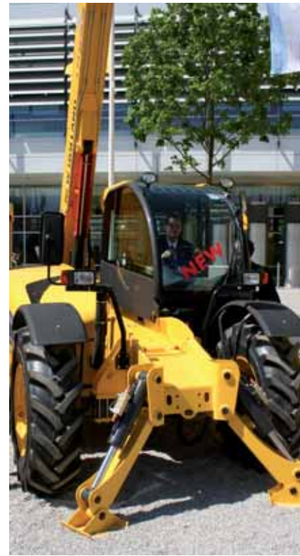
Latest New Holland is the LM1133 which can lift 2.5 tonnes to its maximum 13 metre lift height.
