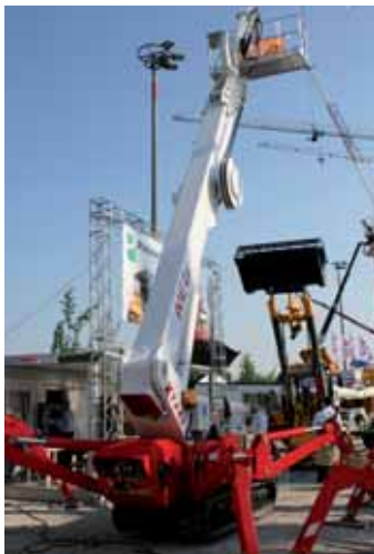
The new XTJ42 has a working height of 42 metres.
