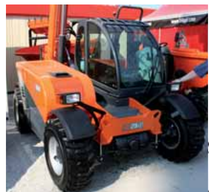
The compact MZ Imer has a 6m, 2.7 tonne lift.
