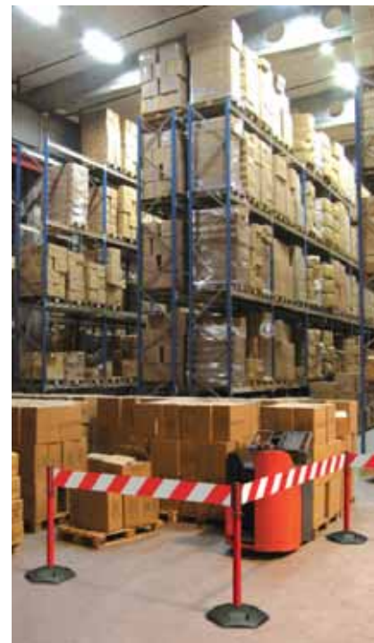
Retractable belt type barriers might be a more efficient way of cordoning-off areas where cranes or lifts are at work?
