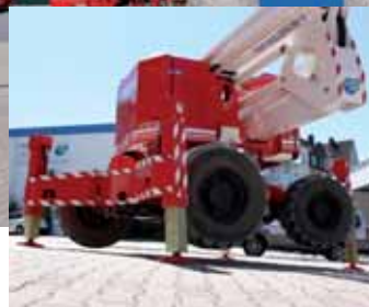
The outriggers on the new Matilsa Parma 21D boom lift provide levelling of up to 17 degrees.
