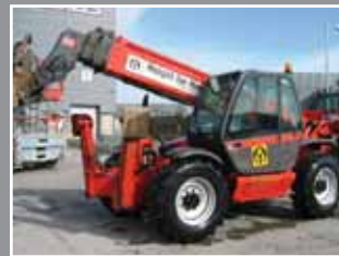
Manitou MT 1740 Telescopic forklift 17m/4 Tonne
