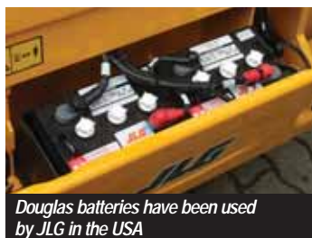
The other big supplier of batteries on new aerial lifts note the quick release filler caps.
