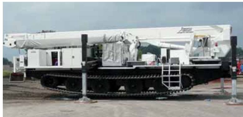
Bronto has placed some of its larger boom lifts on crawler chassis
