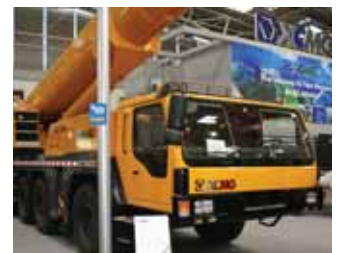
XCMG is China's largest crane producer. This 240 tonne QAY 240 is now part of a range that extends to an eight axle 500 tonner.
