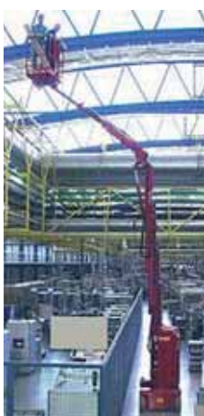
The largest Lehmann machine features 5.15 metres of outreach
