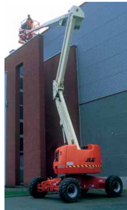
One of several JLG rough terrain machines, the 510AJ has a 15.8 metre platform height and 9.5 metres outreach.
