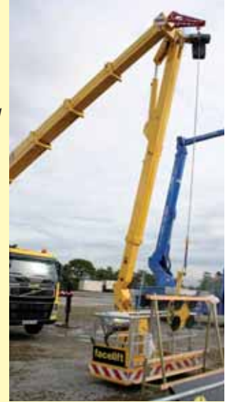
The Ascendant stand sported its all-new 17 metre lift on an Iveco chassis. This new British-built lift incorporates single side outriggers to provide excellent outreach in a small footprint.
