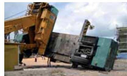
One outrigger punched through the ground.
