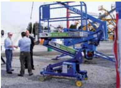
CTE and Planet Platforms launched the new Power Tower, the unique push around powered lift that uses a sigma type linkage to provide a five metre working height with 250kg lift capacity. CTE also showed its new CS179 spider lift and its 19 metre Z19 sigma linkage and telescopic boom truck mount. Planet also displayed the new TP9000 trailer mounted scissor lift.
