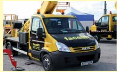
The Ascendant stand sported its all-new 17 metre lift on an Iveco chassis. This new British-built lift incorporates single side outriggers to provide excellent outreach in a small footprint.
