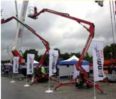
Another new spider lift was to be found on the Promax stand where the company had the new 15 metre Platform Basket 15.75. Designed to pass through a single door the company reported sales from the stand.
