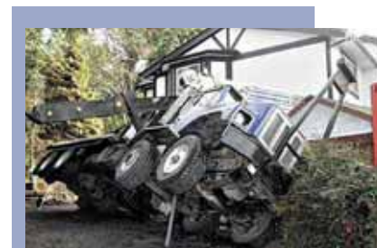
November 2006 - Victoria Canada - An 18 tonne boom truck lifting a hot tub over a house into the rear garden, tipped over when one of its outriggers punched through the driveway into an old septic tank. The tub dropped striking Johnson and placing him into intensive care. The roof of the house was also badly damaged.
