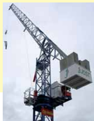
Jost distributor MTI launched the new Jost 68.4 flat top hydraulic luffing jib tower crane. The new crane has a 40 metre jib with a jib tip capacity of 1,500kg and a maximum lift capacity of four tonnes. The unit on show was sold to City Lifting.
