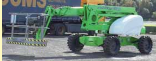
Niftylift showed off its new HR21 4x4 articulated boom lift which is now available with a bi-Energy power pack as well as its most popular models the 12 metre working height HR12 bi-energy and the T120 trailer lift.
