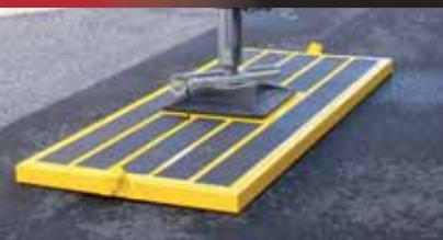
A superb steel outrigger mat on Eisele's new 103 metre Wumag WT1000.
