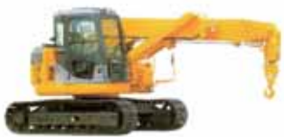
The Maeda LC1385M-2 has a 16 metre boom that can lift 2.6 tonnes to full height.
