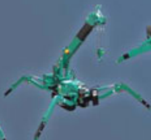
MC285 - 2.8 Ton Mini Crane Capacity (kg/m): 2820/1.4 Max Radius (m): 8.21 Max Height (m): 8.70 Engine: Diesel / Electric
