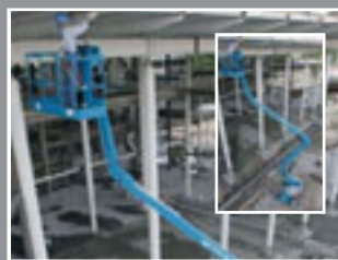
Genie Z51/30 Articulated Boom 17.6m - 2004/5/6/7
