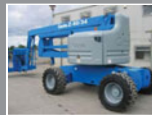
Genie Z60/34 Articulated Boom 20.4m - 2004/5/6/7
