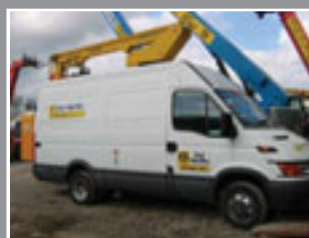
GSR 12.5RA (Iveco) Truck mount 12.5m - 2003
