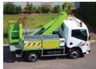
The France Elevateur Topy has 11 metres working height and can carry up to 500kg. This is the electric eco version with solar panels to help recharge the battery.
