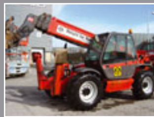
Manitou MT 1740 Telesapler 17m/4 Tonnen - 2005/6/7
