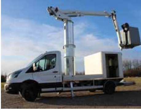
The Danilift PV155V is available on a five tonne truck or van chassis and features a telescopic vertical column which extends to a 4.3 metre up and over height
