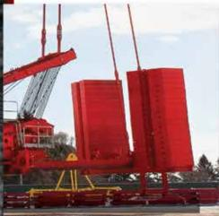
MLC650 with VPC-MAX™ capacity enhancing attachment shown
